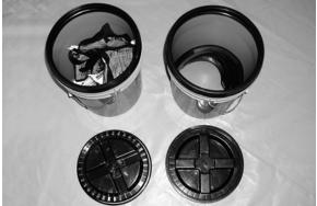
c. Place the rubberized gasket on the lip of one bucket, and place that bucket in the center of the case.
