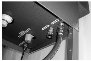
b. Attach the male end of one 25' red hot water hose into the "Hot Input" connector on the bottom of the sink.
