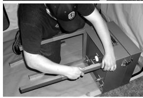
e. Reopen the sink unit and lock support struts into position.
