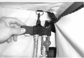
c. Hang the spray nozzle on the black plastic D-ring on the divider wall, below the manifold
