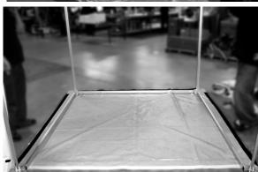
At each of the outside corners, thread the black web strap through it's D-ring and pull snug to form a berm around the frame.
