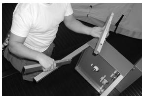
Slide the legs into position in the bottom corners of the sink unit. (Note the legs friction-lock into the sink unit; they do not "snap" into place.)
