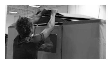
Lay the entryway roof panel on shelter floor and fold as shown.
