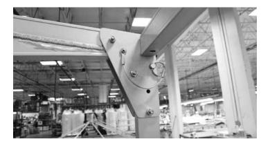
Fold end frame assembly legs and secure with attached black strap.
