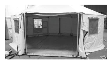
Release the black floor berm strap at the shelter leg to lay down the GateKeeper floor.
