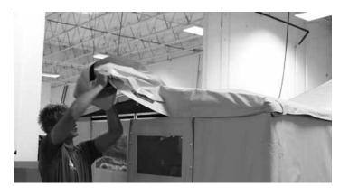
Fold end cap in half two times lengthwise.
